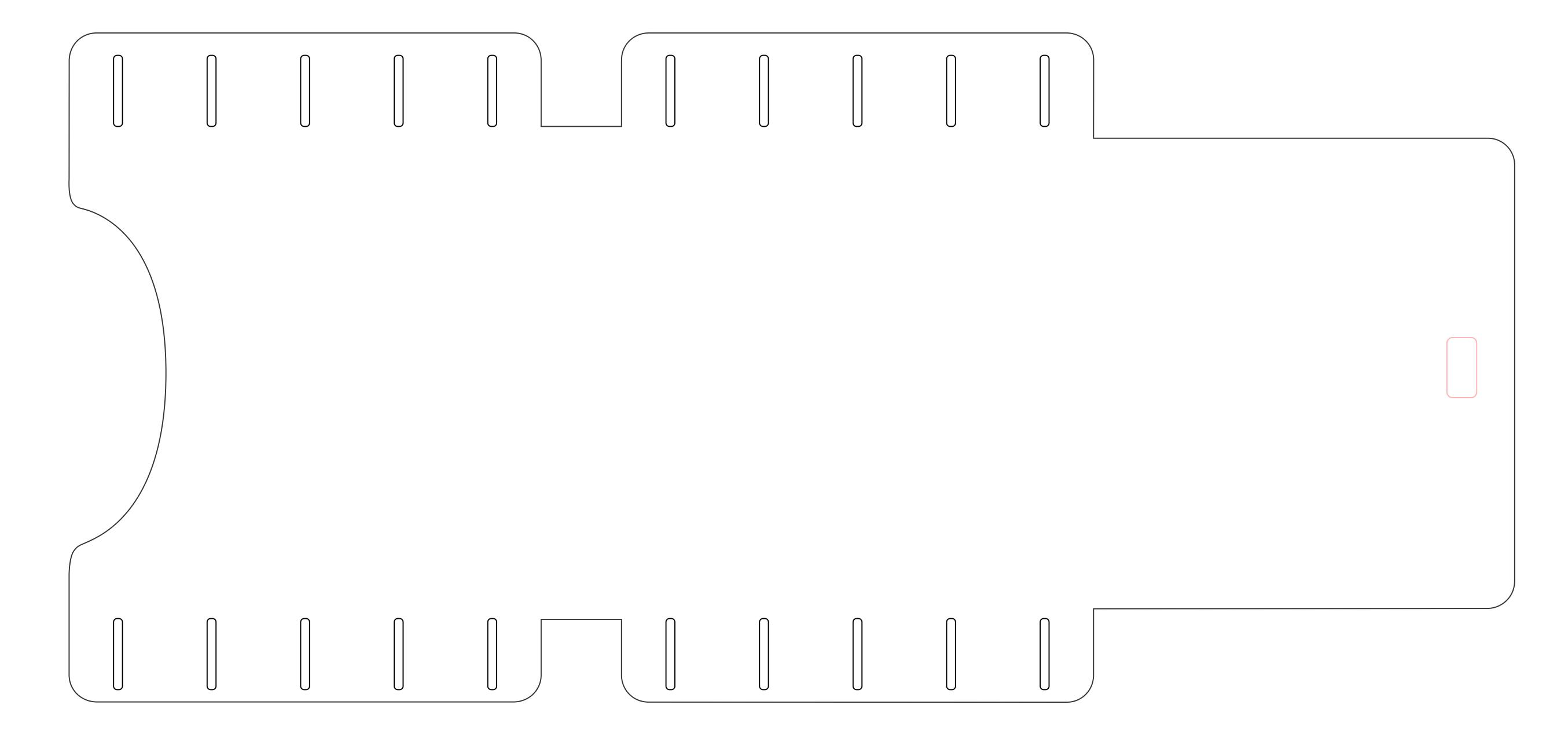
Finished size is about 8.5"X8.5"X1.5" interior Needs 13"x27" leather 1" strapping to finish
